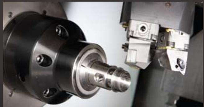
Atomica CNC machines are selected to be the best at the functions they perform. A Titanium first stage body is machined with 23 precision operations in one session.
